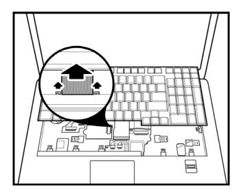
Figure 4-29 Disconnecting the keyboard cable
