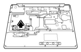
Figure 4-50 Removing the fingerprint module bracket
