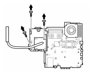
Figure 4-65 Removing the VGA board screws
