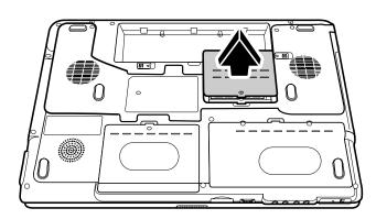
Figure 4-17 Removing the expansion memory module cover
