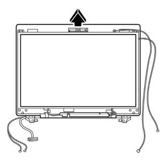
Figure 4-84 Removing the camera module
