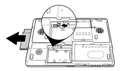
Figure 4-24 Removing the optical drive
