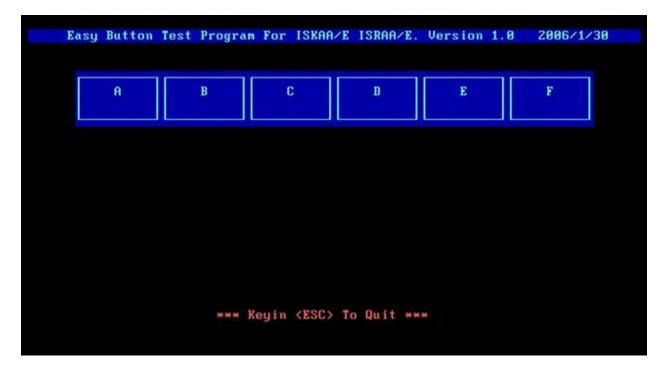
Press each of the buttons on the front panel in turn. A yellow bar will appear on the relevant section of the figure if the button passes the test.
