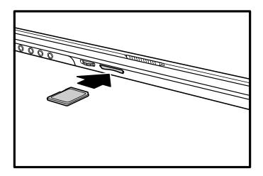
Figure 4-7 Installing the memory card
