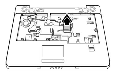
Figure 4-39 Removing the wireless LAN card
