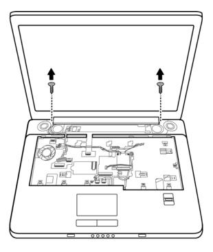
Figure 4-33 Removing the front screws
