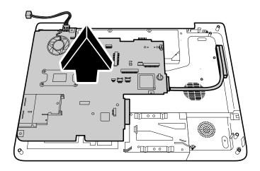
Figure 4-59 Removing the system board
