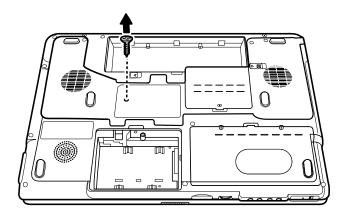
Figure 4-23 Removing the optical drive screw
