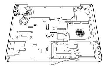
Figure 4-64 Removing the VGA PCB
