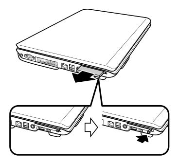
Figure 4-3 Removing the PC card
