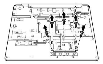
Figure 4-46 Removing the touch pad screw
