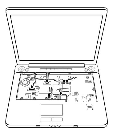
Figure 4-30 Disconnecting cables
