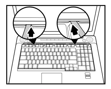
Figure 4-26 Removing the keyboard cover
