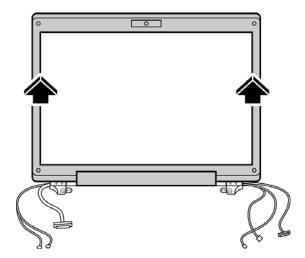
Figure 4-75 Removing the display mask screws
