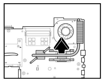
Figure 4-69 Removing the heat sink
