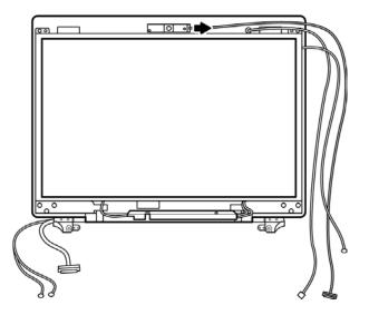
Figure 4-83 Removing the CMOS cable
