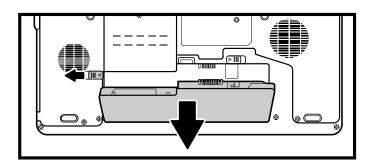
Figure 4-2 Unlocking the battery lock
