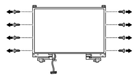
Figure 4-81 Removing the bracket screws
