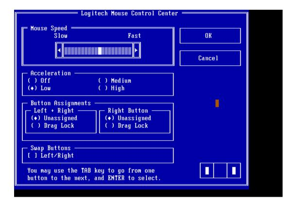
After checking T/Pad buttons and cursor's function, use "Tab" key or use T/Pad cursor to click the "OK" column will end this test.
