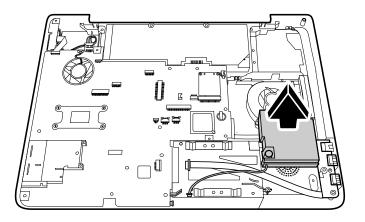
Figure 4-54 Removing the subwoofer unit
