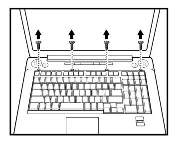
Figure 4-28 Removing the keyboard screws
