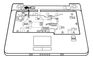
Figure 4-40 Disconnecting the Bluetooth cable
