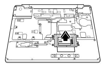
Figure 4-48 Removing the Touch Pad
