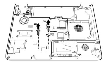
Figure 4-57 Removing the system board screws
