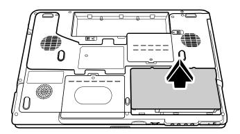
Figure 4-14 Removing the secondary HDD door
