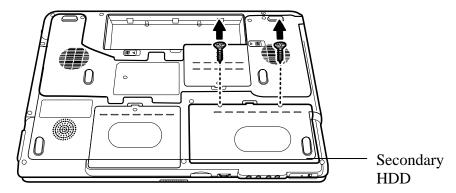
Figure 4-13 Releasing the secondary HDD door screw
