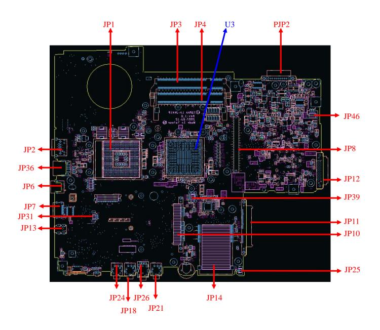
Table B-1 System board connectors (top and bottom)
