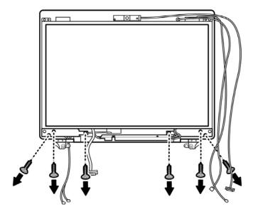
Figure 4-79 Removing the LCD module screws
