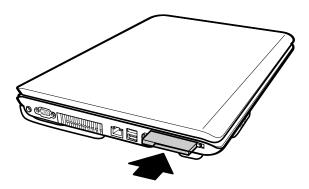
Figure 4-4 Installing the PC card
