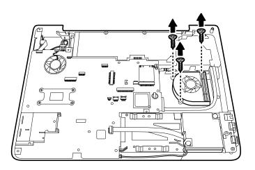
Figure 4-60 Removing the fan screws
