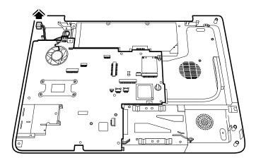
Figure 4-58 Removing the DC power cable
