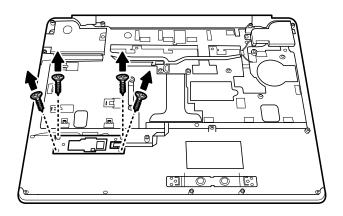
Figure 4-49 Removing the fingerprint module bracket screws
