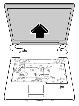
Figure 4-34 Removing the display assembly
