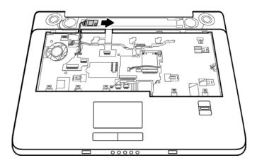
Figure 4-41 Removing the Bluetooth module
