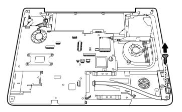
Figure 4-55 Removing the USB board screw
