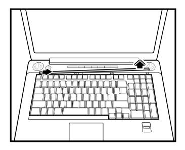
Figure 4-27 Removing the keyboard cover
