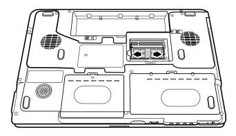
Figure 4-18 Releasing the expansion memory module
