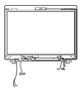
Figure 4-77 Removing the connectors
