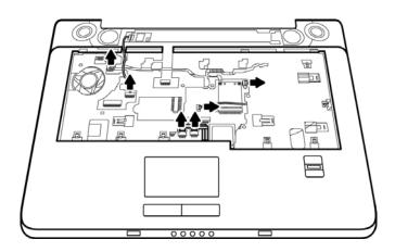
Figure 4-43 Removing the cables
