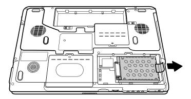
Figure 4-15 Removing the secondary HDD
