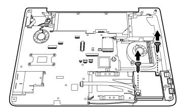
Figure 4-52 Removing the subwoofer screws
