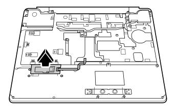
Figure 4-51 Removing the fingerprint module
