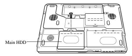
Figure 4-9 Releasing the main HDD door screw
