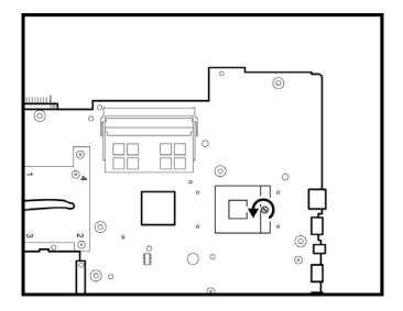
Figure 4-72 Turning the CPU cam
