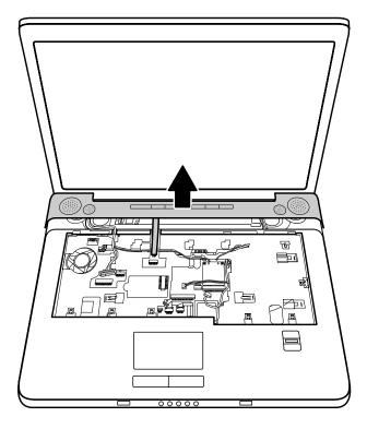
Figure 4-31 Removing the strip cover
