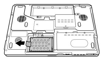
Figure 4-11 Removing the main HDD
