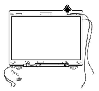
Figure 4-85 Removing the microphone
