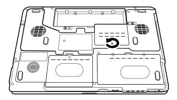
Figure 4-16 Releasing the cover screw
