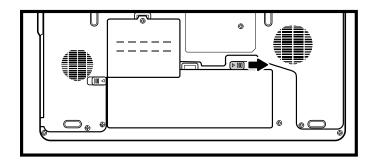
Figure 4-1 Unlocking the battery lock
