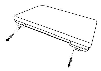
Figure 4-32 Removing the rear screws
