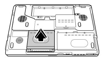
Figure 4-10 Removing the main HDD door
