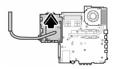
Figure 4-66 Removing the VGA board
