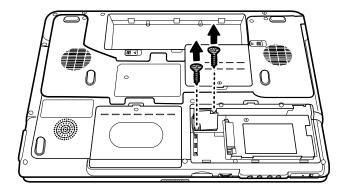
Figure 4-20 Removing the modem module screws
