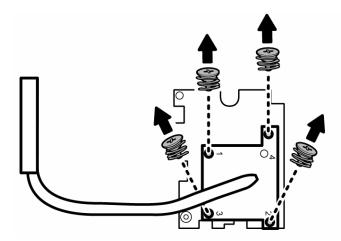
Figure 4-67 Removing the VGA heat sink
