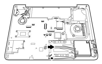
Figure 4-53 Disconnecting the USB board cable and subwoofer cable
