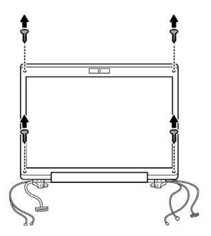
Figure 4-74 Removing the display mask screws
