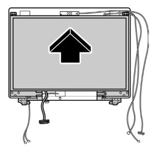
Figure 4-80 Removing the LCD Module
