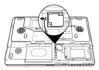
Figure 4-21 Removing the modem connector
