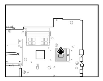
Figure 4-73 Removing the CPU
