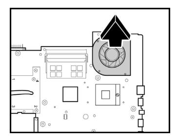
Figure 4-71 Removing the fan
