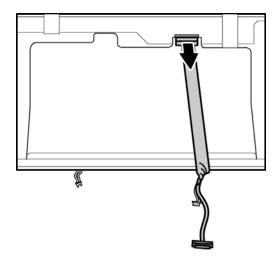
Figure 4-82 Removing the LVDS cable
