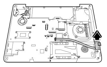
Figure 4-56 Removing the USB board
