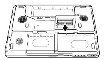
Figure 4-19 Removing the expansion memory module
