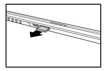
Figure 4-6 Removing the memory card
