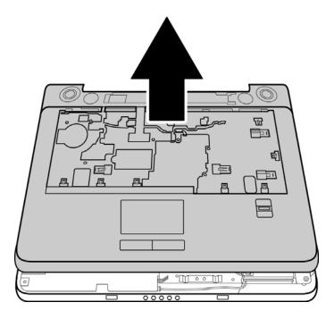
Figure 4-45 Removing the top cover
