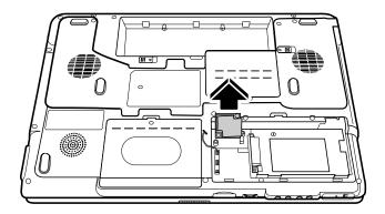
Figure 4-22 Removing the modem module
