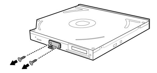
Figure 4-25 Removing the optical drive bracket
