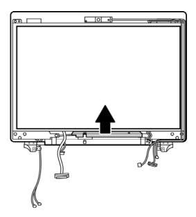
Figure 4-78 Removing the FL inverter board
