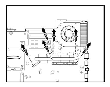
Figure 4-68 Removing the heat sink screws
